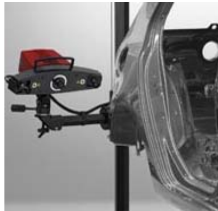
Figure 1. ATOS non-contact laser scanning system
