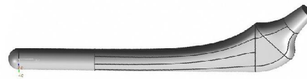
Figure 11. Solid model of a femoral stem built by Unigraphics NX. (Type II)
