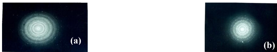
Fig. 7. An electron diffraction pattern indicating (a) before (b) after annealing \text{Bi}_2\text{Te}_3 thin films.
