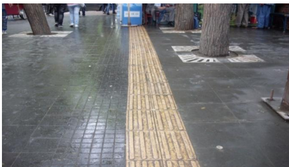
Fig. 5 In these images, you can see the band which helps the blind people to find their directions. However, the band above is blocked by a buffet http://studyofintroductiontoarchitecture.blogspot.com
