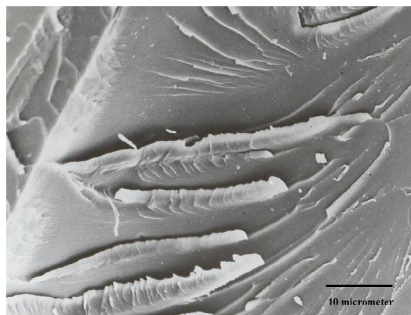
Figure 2. SEM of neat epoxy without Hycar
