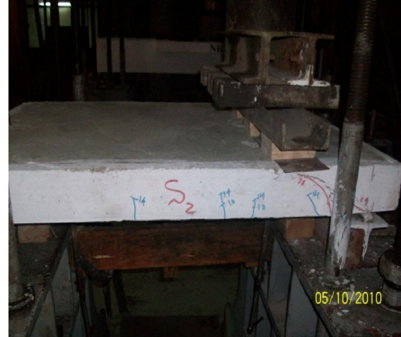
Figure (5): Shear failure of slab S2
