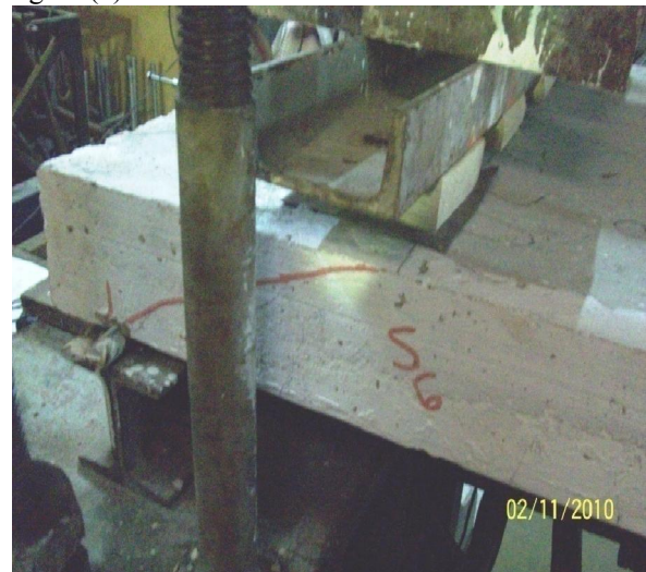
Figure (9): Shear failure of pre-slab S6
