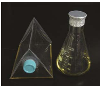
Figure 2. The flexible Celloom reactor vs glass flask
