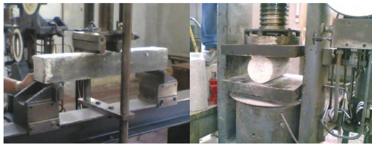
Fig. 6: Plain Concrete Beam and Concrete Cylinders under Test
