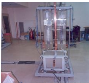
Figure 2, Electrolysis with 5 kw and Nominal production capacity 1 normal m/hr hydrogen
