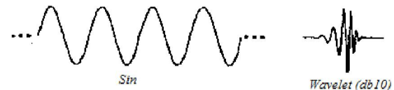
Figure 1. Comparison of wavelet and pure sinusoidal waveforms [17]
