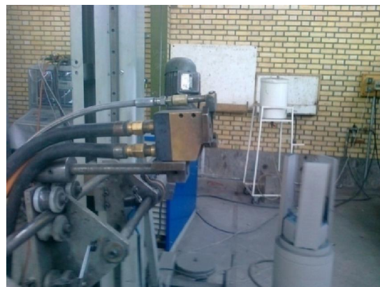
Figure 4. Plasma spray gun on samples for molybdenum coat creation
