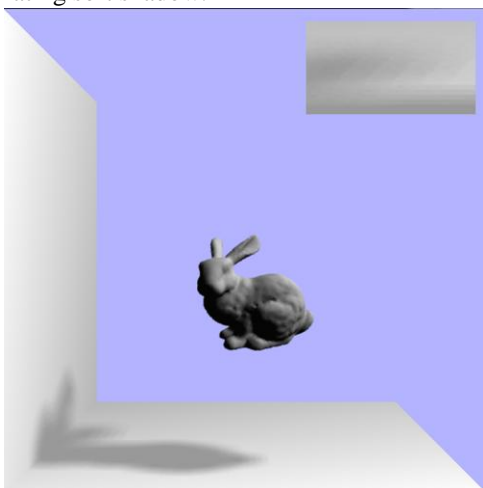
Figure 9. Result of soft projection shadow with 360 samples using simple sampling and stencil buffer.
